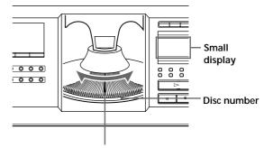
Disc slot at the loading position
